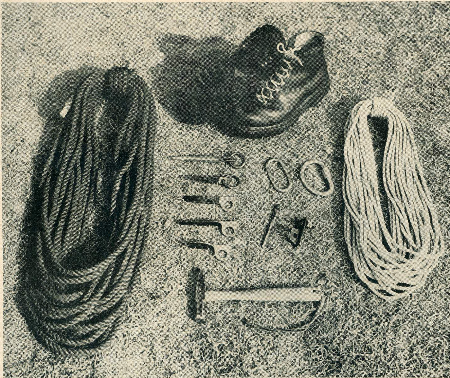
Equipment used in the climb of Shiprock included 7/16 inch nylon climbing rope, 1/4 inch nylon climbing rope, Bramani soled climbing boots, piton hammer, assorted types of pitons (center), two types of karabiners (upper left center), and an expansion bolt assembly with an expansion bolt drill (upper right center). The group was equipped with seven ropes of over 100 feet each, eight expansion bolts, 50 pitons and 15 karabiners.
