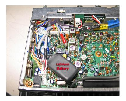
Icom IC-28A bottom circuit board showing the lithium battery wrapped in shrink tubing. The red and white wires at the top coming out of the front panel are the wires to the new pot.
