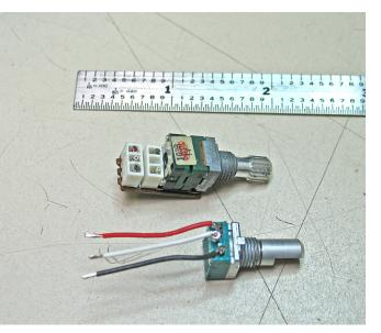
**CHK Function**: This function allowed the user to see the transmit frequency when in Duplex or repeater mode. Since I could not find a pot with a push button switch this function is lost. Much of my operation is mobile in simplex mode so I don't need this function anyway.
