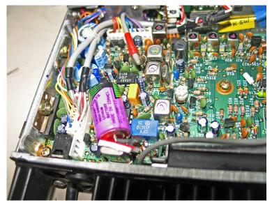
TADIRANS THE IN LEASE WILL IN ISRREL COMPANY THE INTIAL The new battery in place.
